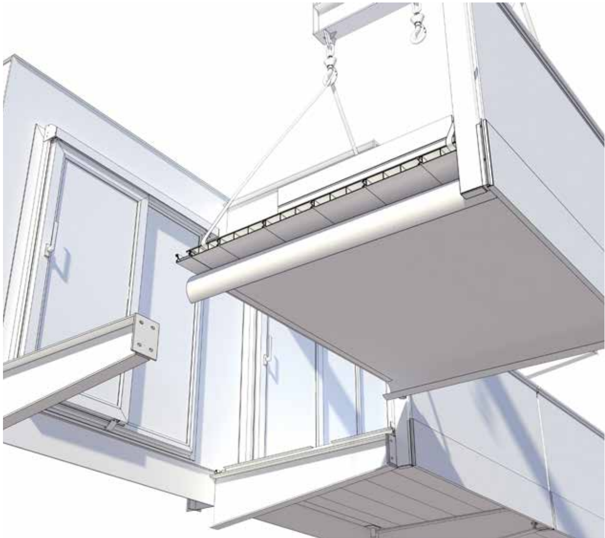
Pre-assembled balcony units are lifted and secured in place within minutes.
